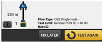
Link with an APC connector shown as a loss event
